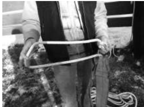
2. Similar to the one man diamond make a loop long enough to toss over the center of the load (about 8' long).
