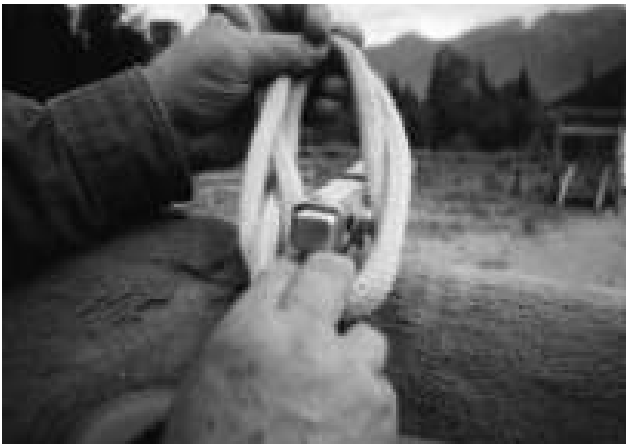
This clove hitch is securing a basket rope on the forks of a modern adjustable sawbuck.
